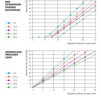
Bed expansion and pressure loss curves are provided for the most commonly used particle water. Charts are available for all particle sizes on request, and for fluids of various viscosities
